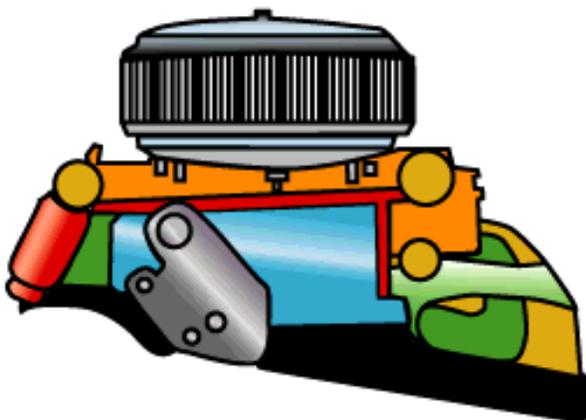
Fuel injected engines without carburetors require a backfire flame arrester over the air intake to prevent exhaust valves from backfiring into the air chamber which might cause a fire or explosion.
